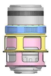
5. The tightness between the SA Control ring gear and the lens can be adjusted by removing rubber grips on either sides of the plastic C-ring.
