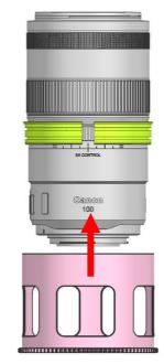
2. Insert the SA Control ring gear on the plastic C-ring until it reaches the flange of the plastic C-ring.
