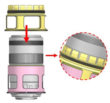
3. Insert the CRF100-F\_Focus gear as shown and place it over the lens
