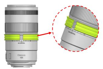
1. Insert the plastic C-ring for SA Control ring gear as shown and place it over the lens
