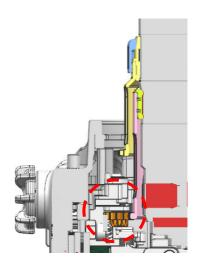
2. The SA Control ring gear can be controlled through Control ring mount adaptor Fn of the housing [Front dial]
