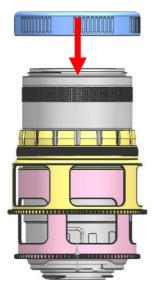
4. Place the Locking Ring for CRF100-F\_Focus gear over the gear, and screw it into the thread on the gear
